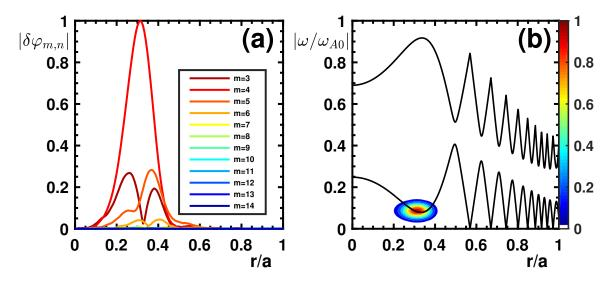
FIG. 4. Radial structures of each poloidal harmonics of scalar potential fluctuations (a) and the corresponding power spectrum in the  $(r,\omega)$  plane (b) are shown in arbitrary units for the n=4 reference case in the central core region. The solid lines in figure (b) represent SAW continuum.
