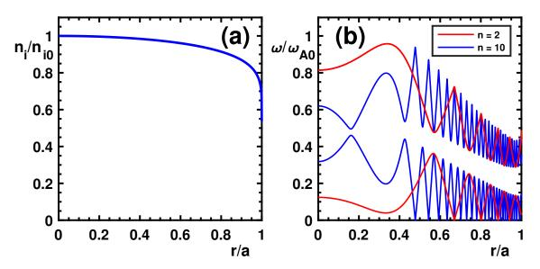
FIG. 2. Radial profile of bulk ion density  $n_i$  normalized to its on-axis value  $n_{i0}$  (a) and the shear Alfvén continua for two typical mode numbers n = 2 and n = 10 (b).
