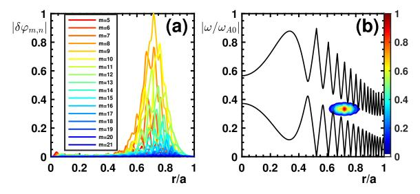
FIG. 12. Analogous to Fig. 4, radial structures of each poloidal harmonics of scalar potential fluctuations (a) and the corresponding power spectrum in the  $(r,\omega)$  plane (b) are shown in arbitrary units for the n=6 reference case in the outer core region. The solid lines in figure (b) represent the SAW continuum.
