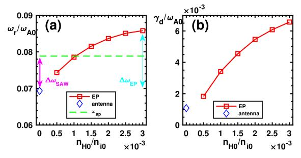
FIG. 6. RSAE real frequencies  $\omega_r$  (a) and damping rates  $\gamma_d$  (b) from the EP density scan, the respective values in the MHD limit  $(n_{H0}/n_{i0}=0)$  measured by antenna are also included. In addition, the RSAE accumulation point  $\omega_{\rm ap}$  is shown as a green dashed line in figure (a).
