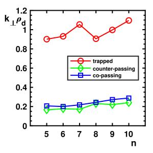
FIG. 18. Numerical calculations of  $k_{\perp}\rho_d$  with respect to n, with  $\rho_d$  representing the banana orbit width of trapped particles and drift orbit width of passing particles. Here,  $k_{\perp}$  and the banana orbit width of trapped particles are measured as in Fig. 10, while the drift orbit width of passing particles is measured for resonant test particles, including the correction due to finite Shafranov shift.
