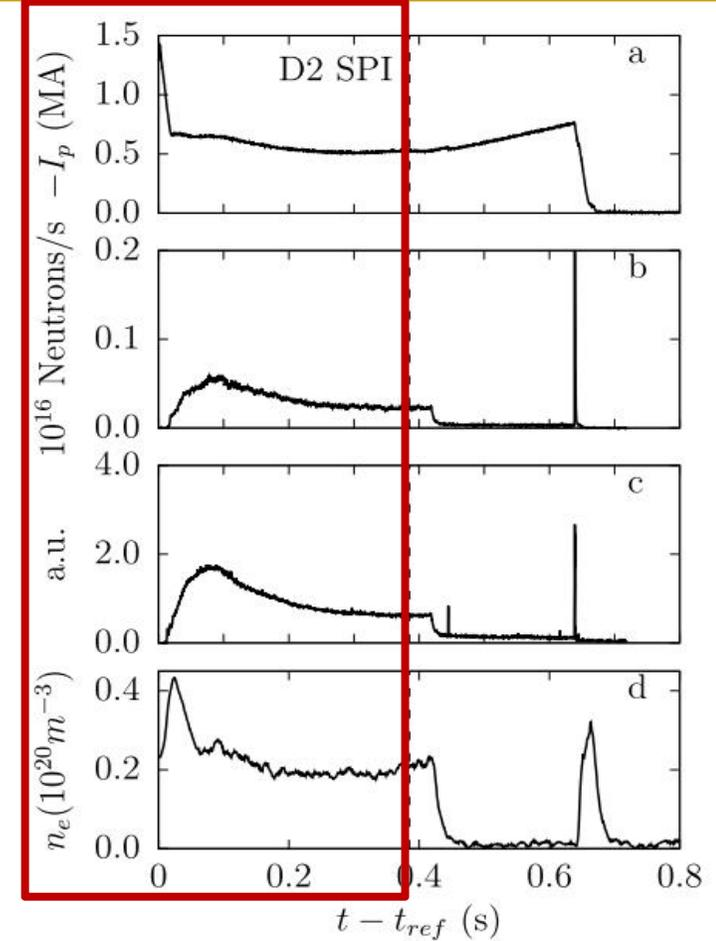
**Figure 1.** Time traces of (a) plasma current, (b) neutron rate, (c) HXR signal, and (d) line-averaged electron density from the experimental shot #95135. The time corresponding to  $t_{ref} = 48.0233$  s in the discharge is taken as reference. The dashed vertical line represents the instant of  $D_2$  SPI.
