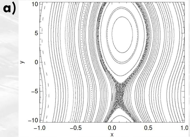
□ **Poincarè maps** of the magnetic field lines show the **topology of the magnetic field on the sections  $z = \text{const}$**
