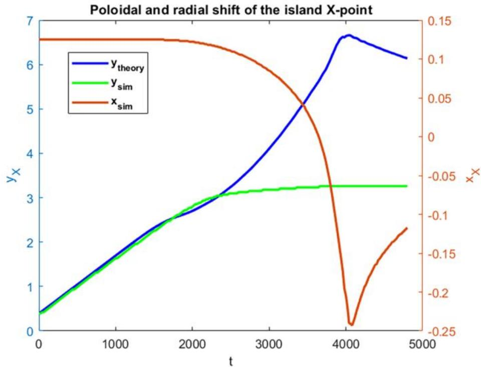
**FIG. 14.** Temporal evolution of the X-point position of the magnetic island in the case  $\eta = 1 \times 10^{-4}$ ,  $c/v_A = 1$ , and  $\Delta' = 6.057$ ,  $d_e = 0$ ,  $\rho_s = 0$ . The green line shows the numerical poloidal shift, while the blue line corresponds to the theoretical prediction according to the formula (15). The rust line represents the displacement along the x direction.
