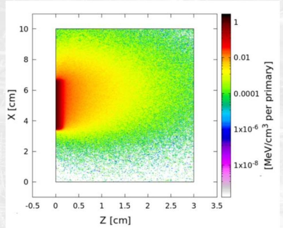
2D projection of the ED on the XZ plane for W at the right panel with a point beam impacting at  $(X,Y,Z)=(5,5,0)$  cm with 5 degrees impact angle with respect to the X direction
