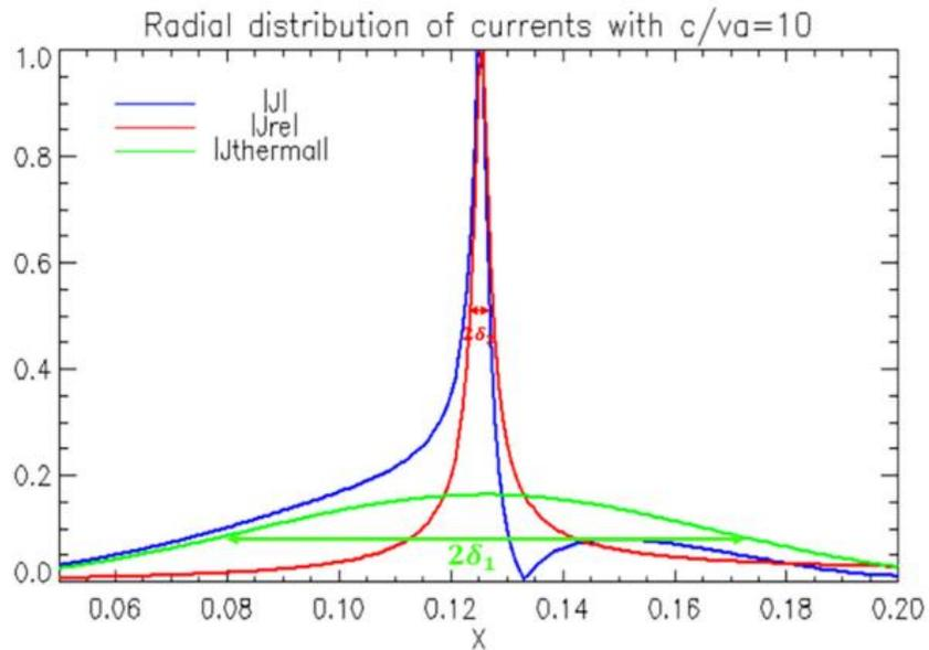
FIG. 6. Eigenfunction of mode 1 for total current (blue curve), runaway current (red curve), and thermal electrons current (green curve) profiles showing the inner layer  $\delta_2$  on the runaway current profile and the resistive layer  $\delta_1$  on the thermal electrons profile for  $\eta = 1 \times 10^{-4}$ ,  $\Delta' = 6.057$  and  $c/v_A = 10$ ,  $d_e = 0$ , and  $\rho_s = 0$ .
