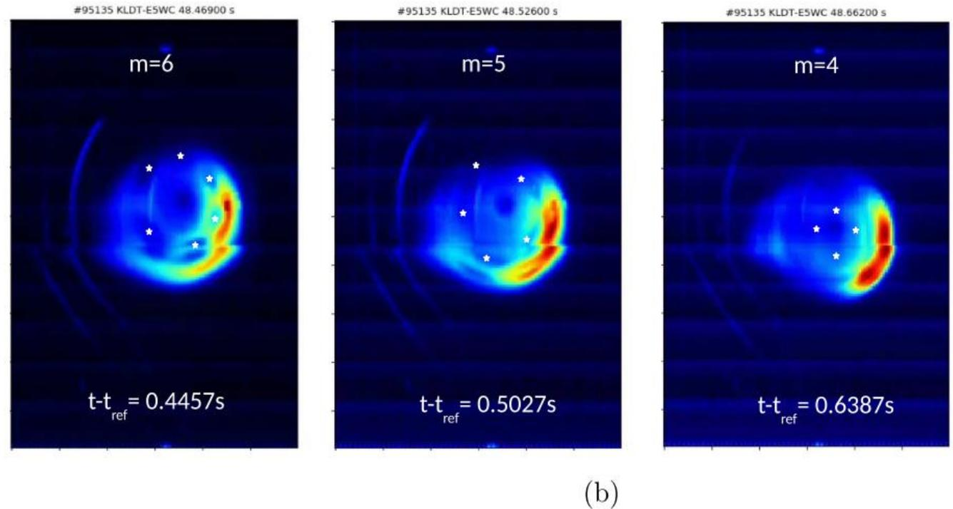
(a) Approximate minor radial location of magnetic structures at various time points until the final crash. (b) Synchrotron images showing the magnetic structures, highlighted by the 'star' symbols.
