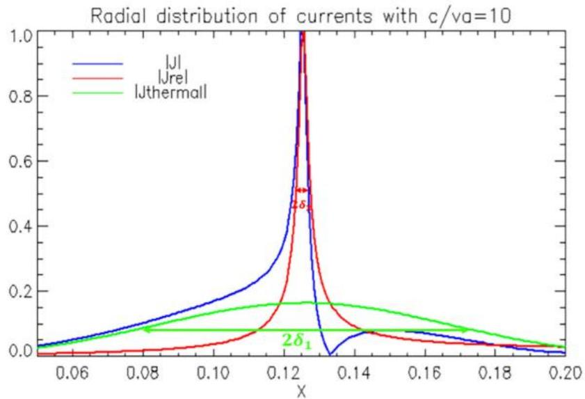
**FIG. 6.** Eigenfunction of mode 1 for total current (blue curve), runaway current (red curve), and thermal electrons current (green curve) profiles showing the inner layer  $\delta_2$  on the runaway current profile and the resistive layer  $\delta_1$  on the thermal electrons profile for  $\eta = 1 \times 10^{-4}$ ,  $\Delta' = 6.057$  and  $c/v_A = 10$ ,  $d_e = 0$ , and  $\rho_s = 0$ .
