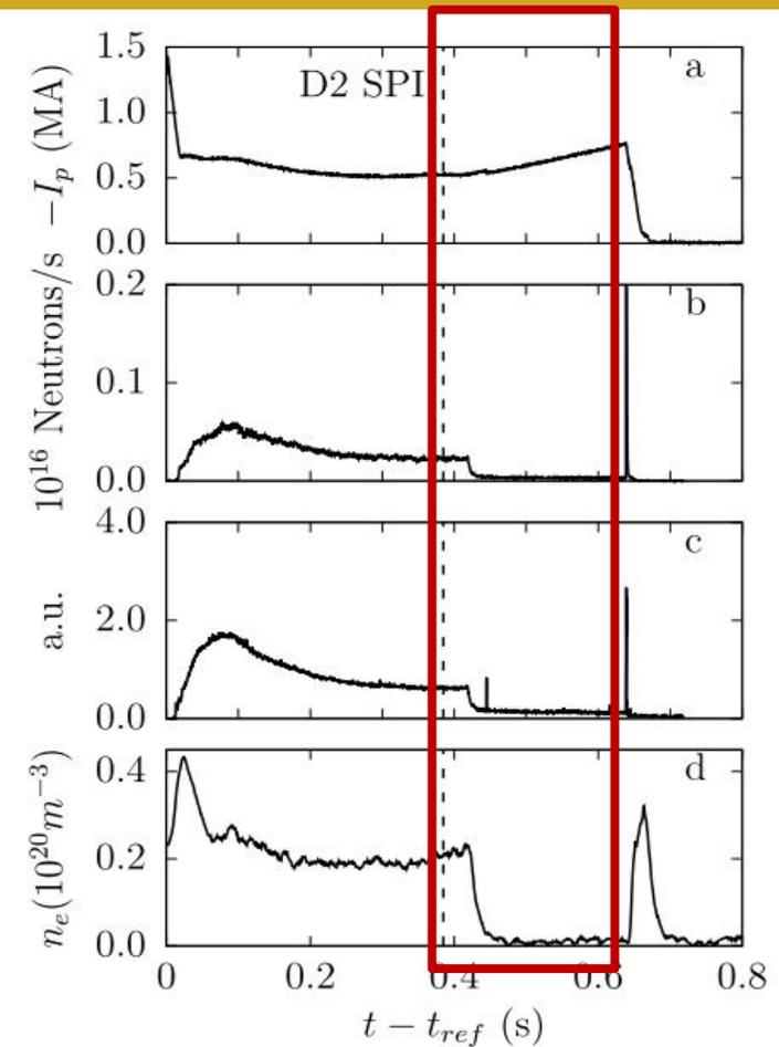
**Figure 1.** Time traces of (a) plasma current, (b) neutron rate, (c) HXR signal, and (d) line-averaged electron density from the experimental shot #95135. The time corresponding to  $t_{ref} = 48.0233$  s in the discharge is taken as reference. The dashed vertical line represents the instant of  $D_2$  SPI.
