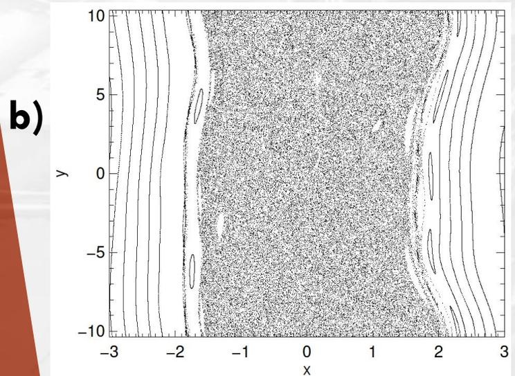
□ In the nonlinear phase (b) of the evolution, **multiple helicity modes with comparable amplitude coexist**. Their interaction leads to the **global stochastization of the domain**
