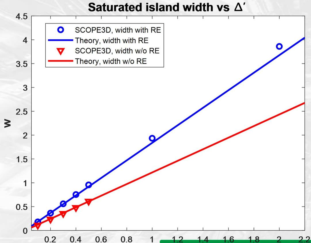
□ The magnetic island width at saturation is around 50% higher in the presence of RE. In addition, no divergence is seen with increasing  $\Delta'$  remaining always in the small  $\Delta'$  regime.
