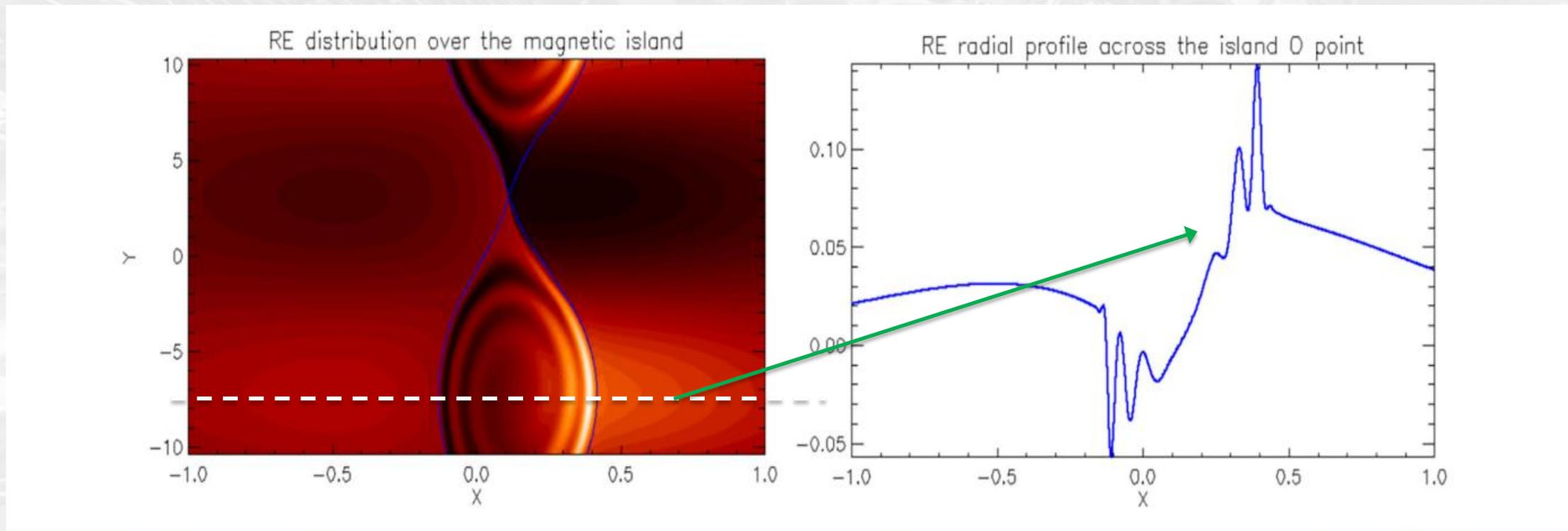
**FIG. 13.** Distribution of the perturbed runaway electrons current with the corresponding magnetic island (blue line) during the nonlinear phase (left) and RE profile (right) at  $t = 2500$  across the island O-point for  $\eta = 1 \times 10^{-4}$ ,  $c/v_A = 1$ , and  $\Delta' = 6.057$ ,  $d_e = 0$ ,  $\rho_s = 0$ .
