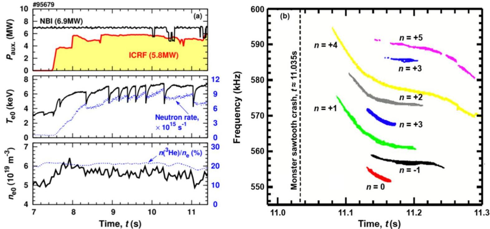
**Figure 1.** (a) Overview of JET pulse #95679 (3.7 T/2.5 MA) in D-<sup>3</sup>He plasmas with energetic D-ions and fusion-born alpha particles. (b) Dynamics of Alfvén activities in the EAE frequency range after the monster sawtooth crash at  $t \approx 11.035$  s.
