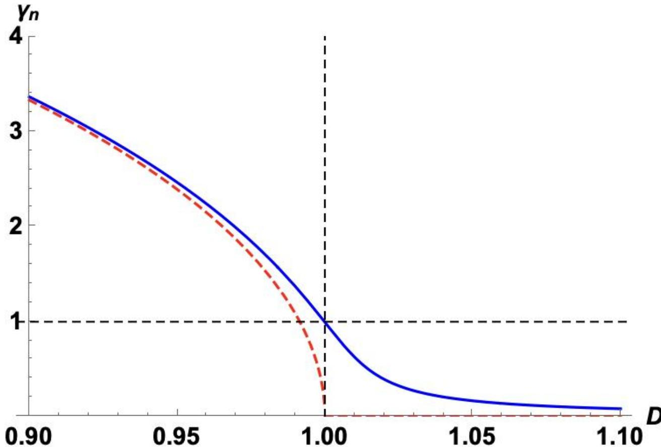
Growth rate  $\gamma_n = \gamma(D)/\gamma(D = 1)$  for the thin wall limit, with  $\gamma(D = 1)$  given in Eq. (16), as function of the ideal wall parameter  $D$  close to ideal-MHD marginal stability. The blue curve shows the numerical solution of the full cubic dispersion relation (Eq. 13), while the dashed red line represents the ideal wall solution.
