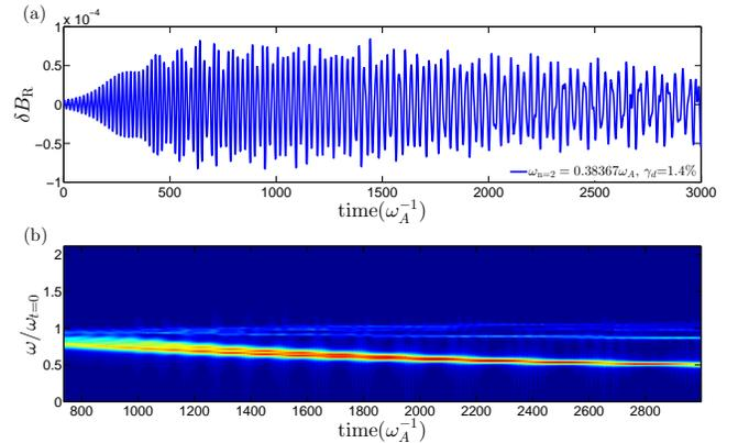
FIG. 2. (a) Time evolutions of the radial perturbed magnetic field and frequency spectrum for the  $n=2$  TAE mode from the single pitch angle ( $\Lambda = 0.50$ ) simulation.
