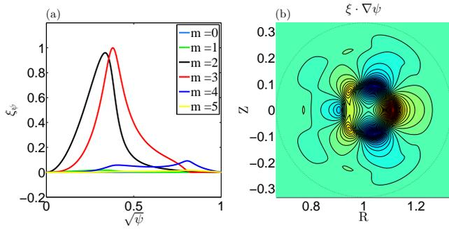
FIG. 1. (a) The  $n=2$  TAE eigenfunction  $\xi_\psi$  and (b) Contour plot of the mode structure  $\xi \cdot \nabla\psi$ .
